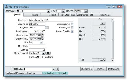
The Bill of Materials module offers a robust set of built-in features. Cost grouping enables you to break down bill of material costs the way you want.
